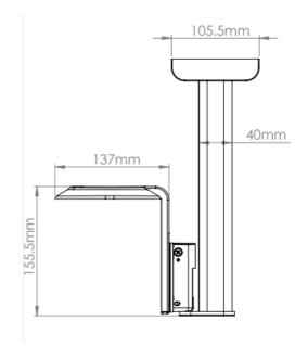
The Flexson Ceiling Mount for Sonos ERA 100 allows you to hang your speaker from the ceiling in the ideal place to sound - and look - great. This new, improved design gives you yet more flexibility and functionality with clever cable routing to the ceiling. It's ideal for commercial installs in bars, restaurants and shops, as well as for home use.
